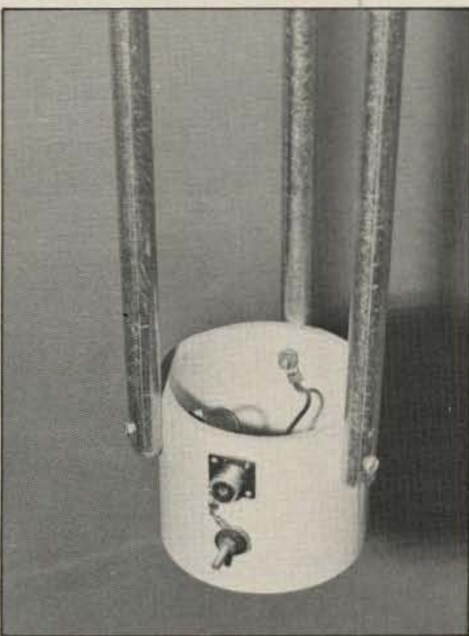
Fig. 4— The base insulator with the SO-239 coax connector mounted on it and wires connecting to the elements. The bolt below is for a ground connection and the radials. A shallow hole can be dug for the base to sit in, or the base can sit on level ground.
